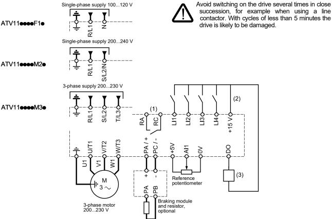
(1) Fault relay contacts, for remote indication of the drive status.
